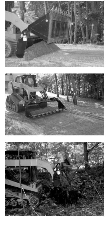
**A WARNING** Lower the attachment to rest flat on the ground, shut down the engine, relieve the hydraulic pressure to the attachment, set the park brake, and wait for all motion to stop before leaving the operator's seat to perform service of any kind.
