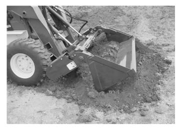
**A CAUTION** Always close the bucket securely before setting the attachment down on the ground. To avoid serious injury or death from crushing, NEVER put any body part near the bucket while open.
